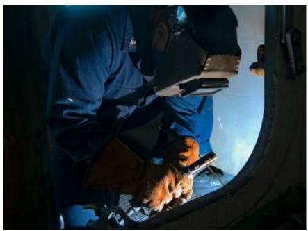
Hull Maintenance Technician 2nd Class Joshua Espinoza, from Houston, welds a bulkhead on a weather deck aboard the Nimitz-class aircraft carrier USS Harry S. Truman (CVN-75) in Portsmouth, Va., on Aug. 7, 2020.
